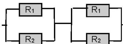
$R_H = \frac{R_1 R_2}{R_1 + R_2} + \frac{R_1 R_2}{R_1 + R_2} = 2 \frac{R_1 R_2}{R_1 + R_2}$
